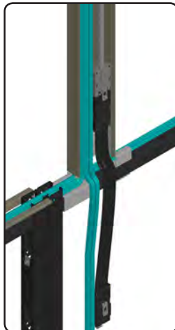
Mount powerpole base bracket 1/4 inch from inside of frame vertical
